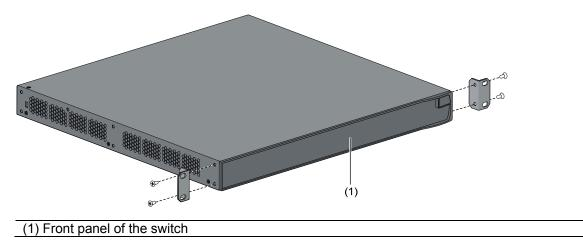
**Step4** Place the switch horizontally in a proper position, and fix the other end of mounting brackets to the front brackets with screws and captive nuts, as shown in <u>Figure 3-5</u>.
